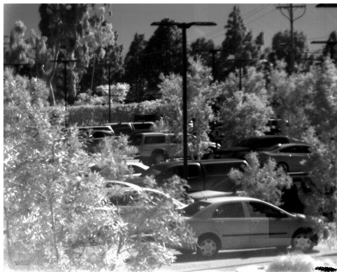
Figure 9 - Picture taken with sensor in LN 2 pour fill dewar heated to 200K.
