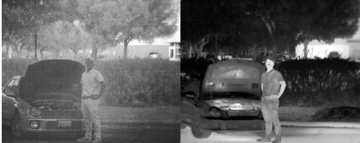
Figure 13 - (left) SWIR and (right) MWIR late dusk imagery from a frame-sequential 1280x1024, 10 \mu\text{m} dual-band SWIR/MWIR with a CTIA and a DI input for the SWIR and MWIR channels, respectively.
