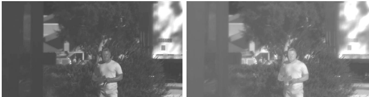
Figure 12 - (left) SWIR and (right) MWIR daytime imagery from a frame-sequential, 1280x720, 8 um dual-band imager with direct injection (DI) inputs for both channels.
