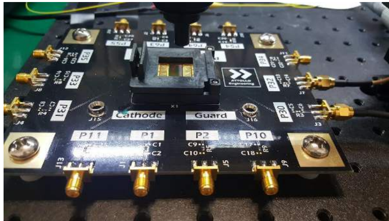
Figure 10. A picture of the Attollo RF performance characterization station showing the fiber focused laser light on the packaged 64-channel detector in an LCC.
