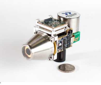
1280x720 with a 8 \mu\text{m} pixel Camera Core
